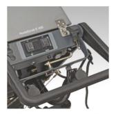
All operational switches are within direct view and easy reach of the operator. Ergonomic handle for operators of any height. Excellent view of the area of be cleaned.
